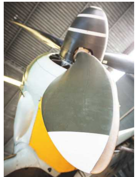
...though the ash, spruce and birch of its propeller are materials familiar to every woodworker
